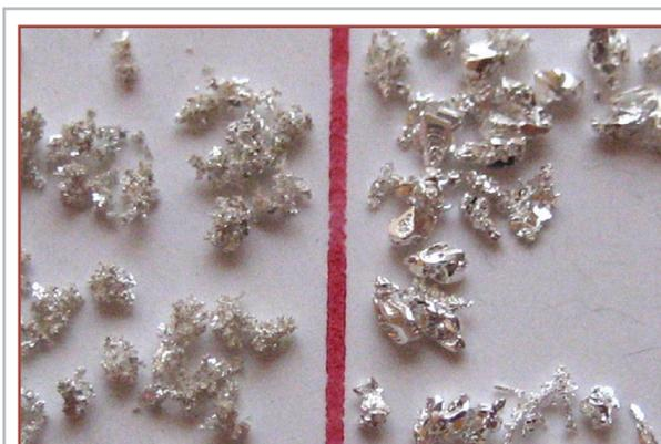
Notice how the rugged surface are of KAR silver crystals on the left side are larger than competitor and vendor E on the right side. (Red line is 0,5mm.)
