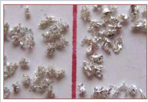
Notice how the rugged surface are of KAR silver crystals on the left side are larger than competitor and vendor E on the right side. (Red line is 0,5mm.)
